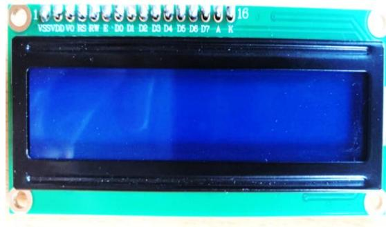
Fig. 4. Physical image of the display
