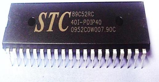
Fig. 3. STC89C52RC MCU physical picture
