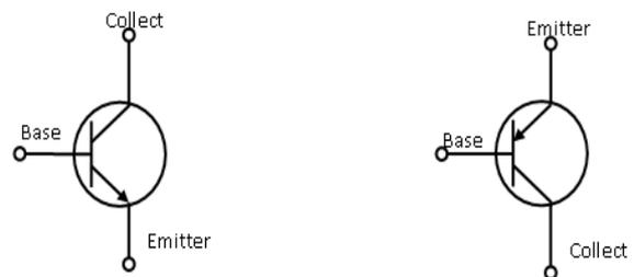
**Fig. 5. Symbol of (a) NPN and (b) PNP transistors**
