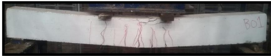
Fig. 7. Crack pattern of control beam B01
